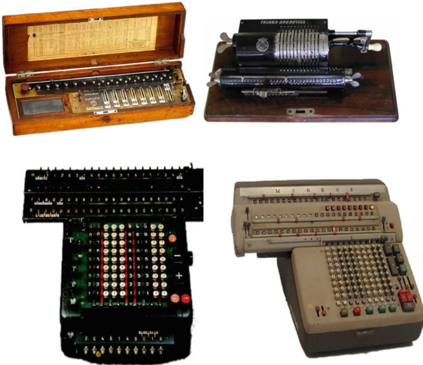
Fig. 5 Mechanical computing devices equipped with the desired capability: Burkhardt Arithmometer , Glashütte, Germany, 1878; Brunsviga , Braunschweig, Germany, 1917; MADAS , Zürich, Switzerland, 1936; (Mult., Automatic Division, Add., Subtr.) MONROE , New Jersey, USA, 1956
