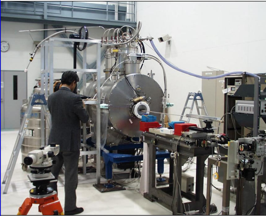
Magnetic field measurements during Site Acceptance Test
